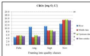
**Fig. 4.4.** Biochemical oxygen demand values in the monitored sections of the Hălçeni Lake
