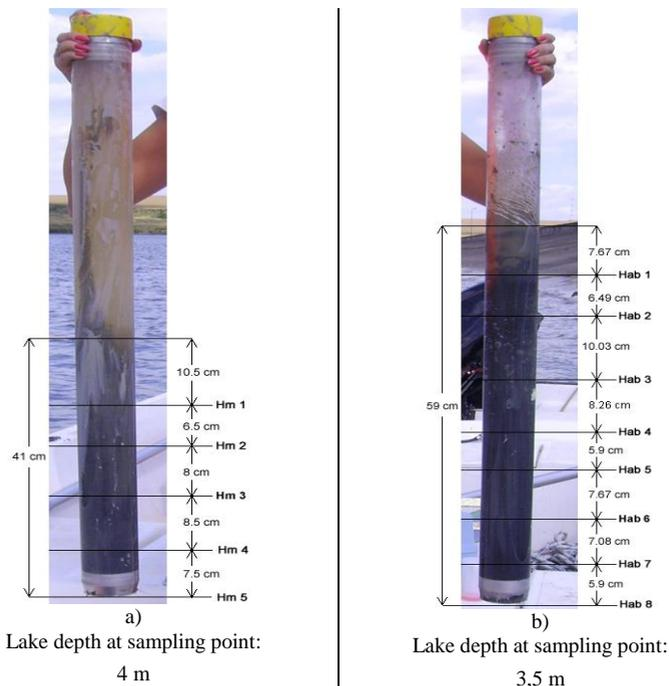
**Fig. 5.1.** Hălçeni Lake, sediment cores from sections: a) *middle lake*, b) *upstream dam*
