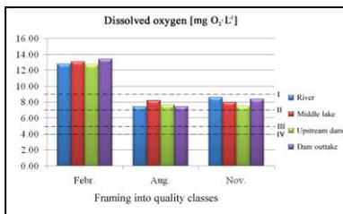
**Fig. 4.3.** Dissolved oxygen values in the monitored sections of the Hălçeni Lake
