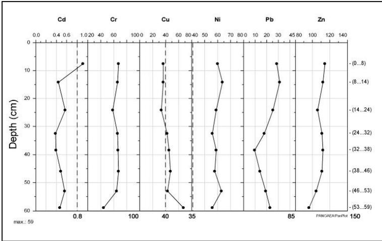
**Fig. 5.3.** Trace element variation for *upstream dam section*, Hälçeni Lake ( $\text{mg}\cdot\text{kg}^{-1}$ )
